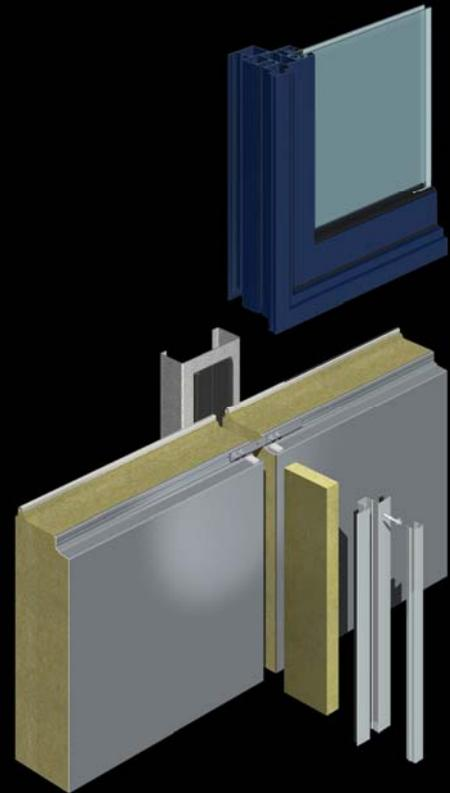
The strength and rigidity afforded by the panel system enable longer unsupported span conditions, reducing the amount of secondary steel work and therefore cost and time on site.
